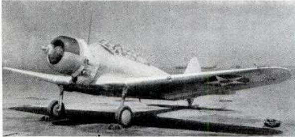
The XBT-2 had a fully retractable landing gear and a larger engine—a Wright Cyclone replacing Pratt & Whitney engine.
