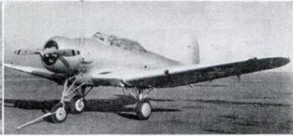
This BT-1 was used for testing a tricycle landing gear that did not prove satisfactory. Landing wheel nacelles are gone.
