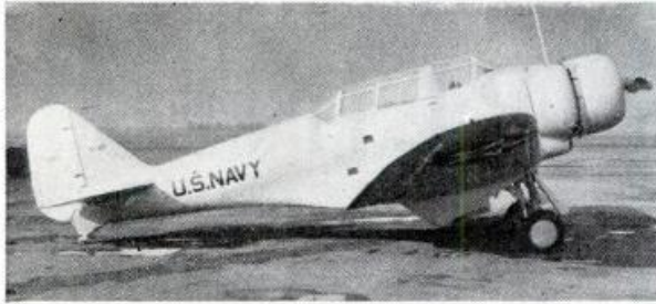
The XBT-1, first of the series. Note especially the extended landing wheel nacelles, the small tail surface, small engine.
